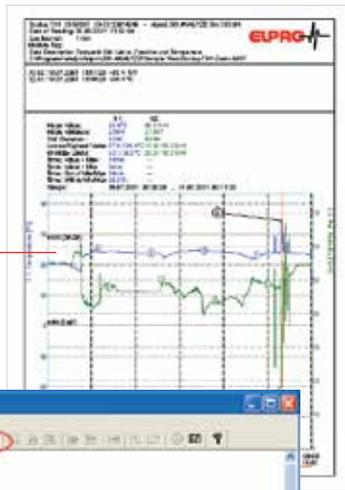
Tabular display with colored text to highlight measured values outside alarm limits.
